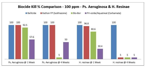
These results show the kill effectiveness of these biocides at the lowest treat rate -100 ppm, which is equivalent to a 1:10000 or 1 oz: 80 gallons volumetric treat rate. From these results, we can see the following:
